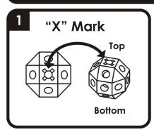
Look on the connector to find the "+" for the top and the bottom of the connector.
