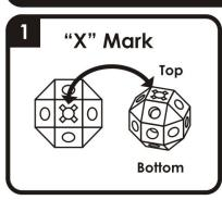
Look on the connector to find the "+" for the top and the bottom of th connector.
